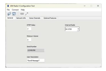
Upon opening the JEM Radio II Configuration Tool you'll be greeted with the General tab where you'll find various settings and information about the JEM Radio II you're connected to.
