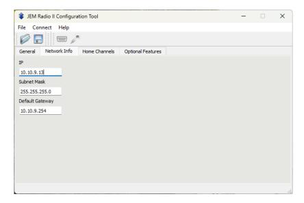
The Network Info tab is where you can view the current IP address of the radio, including Subnet Mask and Default Gateway should you want to connect to the radio via the Network/Ethernet port.
